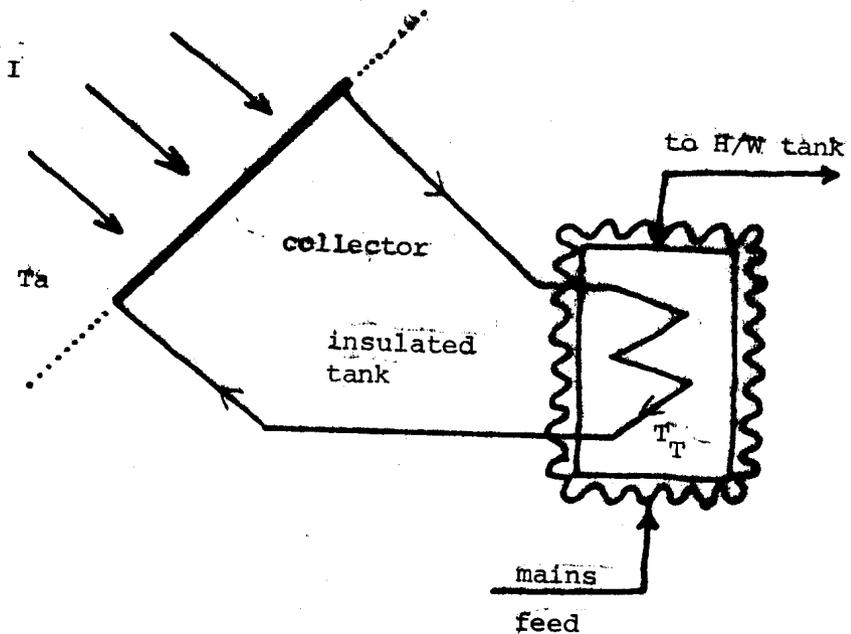
An array of double glazed solar collectors (area  $A_c$ ) is coupled to an insulated water tank (volume  $V_t(l)$ ) by an indirect pumped circuit. The efficiency of the solar collectors ( $\eta_c$ ) is determined by the construction of the collector, the tank temperature ( $T_T(C)$ ), the ambient air temperature ( $T_a(C)$ ) and the incident radiation on the collector surface ( $I(Wm^{-2})$ ), i.e.
