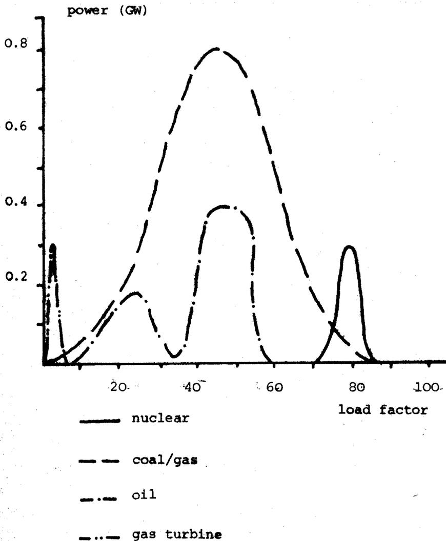
The power is taken incrementally in steps of 250 MW; the merit in steps of 1 GW. Firstly the nuclear is brought on stream, then half the coal, then natural gas, then coal and oil and finally gas turbine (oil fired). This procedure is illustrated in the example below.
